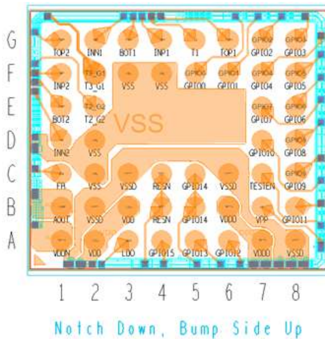
Figure 4: Pin Layout WLCSP
